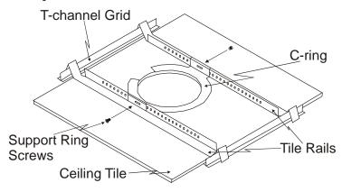
Figure 4: Mounting the SPK-C612
